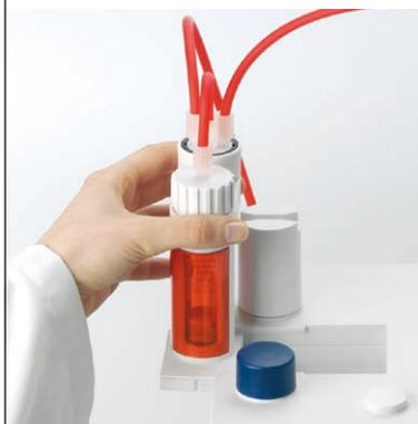
Automatic burette recognition feature ensures that all quality-relevant data such as concentration, titer and expiration date are promptly read in and checked, irrespective of the drives on which the burettes with the titrants are present. The password-protected user management system coupled with user rights guarantees that critical data cannot be changed by mistake.
